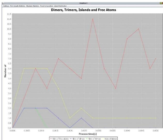
**Figure 15: Time evolution of the number of free atoms, dimers and trimers, and islands during the simulation corresponding to dissolution without evaporation.**
